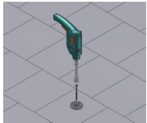
Fig. 7: After filling the hole with sealant, secure the roof shoe with the lag bolt. Tighten to 20 ft. lbs
