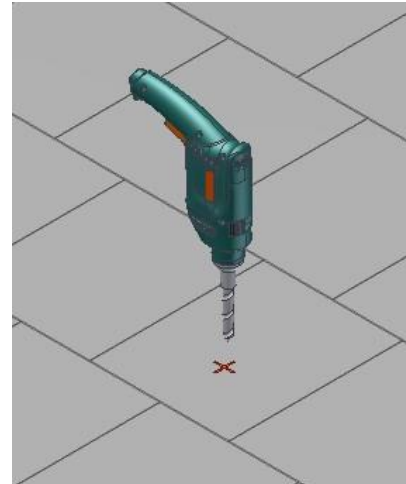
Fig. 6: Locate lag screw mounting. Drill a 7/32" hole through the shingle to a depth of 2 inches
